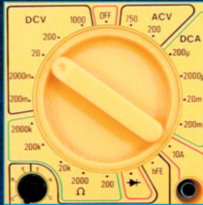
9. The selector switch is used to select which function you want to work with.
